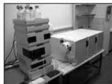
LC-MS/MS Liquid Chromatograph Agilent Technologies 1200 and Triple Quadrupole Agilent Technologies 6410
