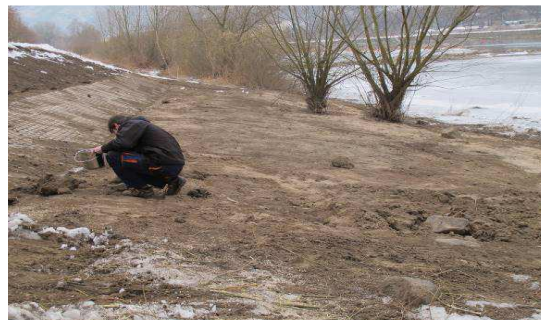
Right bank – after removal of contaminated soil, final sampling
