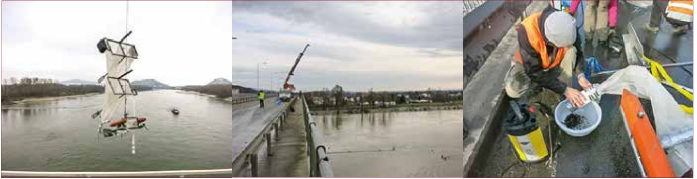
Fig. 2: left picture: the sampling rack with drift nets at three depth stages moments before submerging for sampling; middle picture: lorry with crane during sampling; the rack is submerged in the river, only the upper skimmer is visible at the very right end of the picture; right picture: withdrawal of a sample from the sampling container. C University for Natural Resources and Life Sciences (2014)
